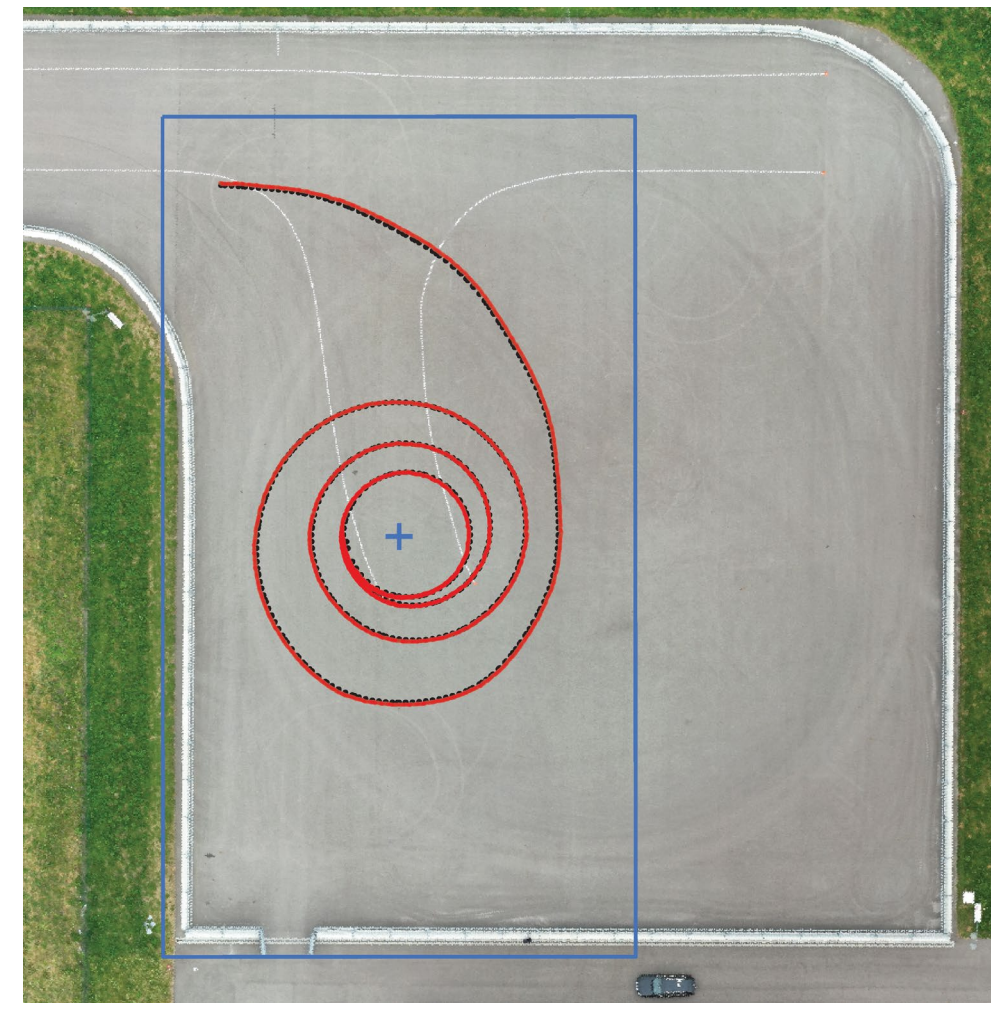
Figure 1: Trajectory driven on test track, black: D-GPS, red: estimation
